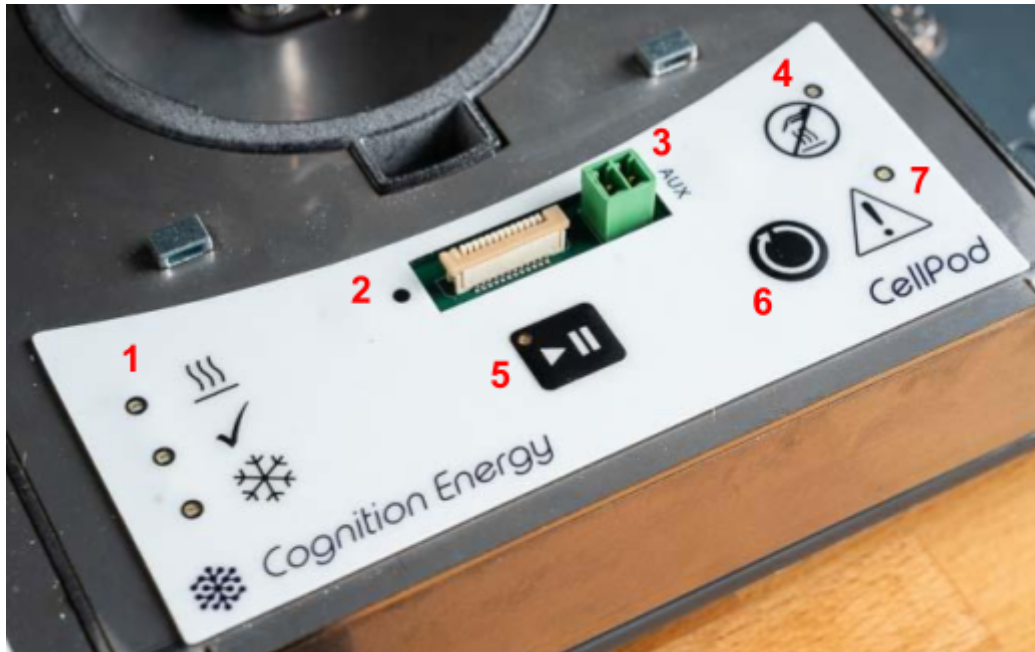
Figure 16: CellPod front panel controls, identifying key features.
