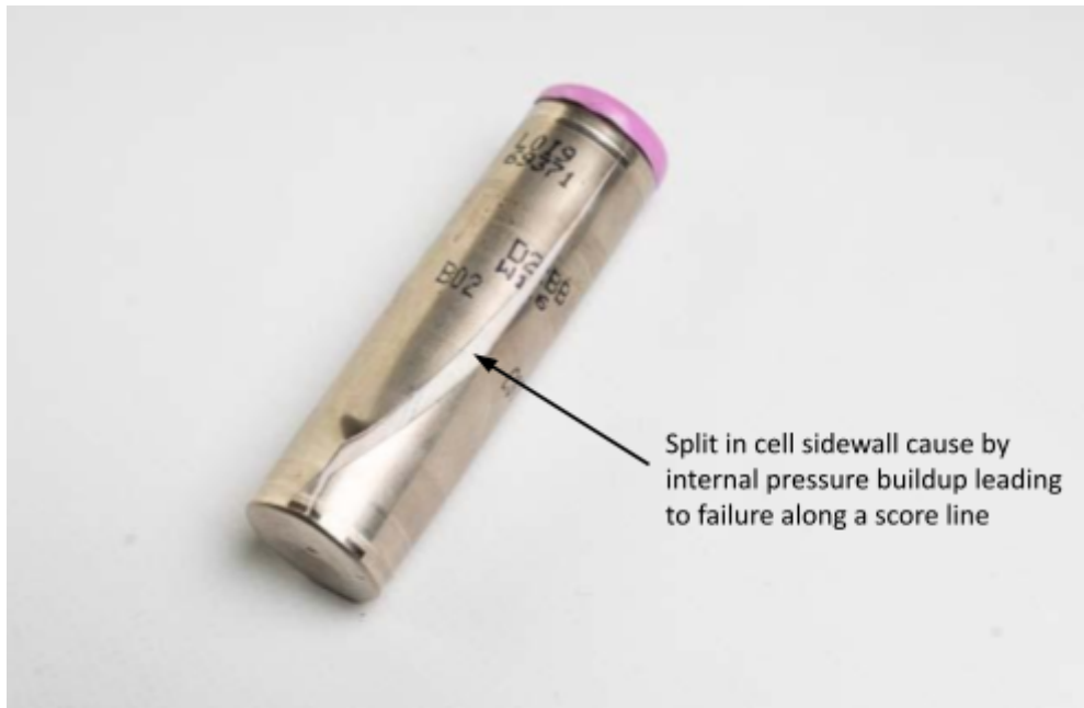
Figure 18: A cell that has split open during cycling due to internal pressure rise and a scratched cell can side wall.
